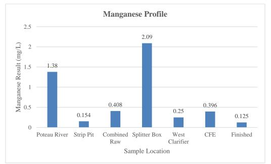
Figure 5: Manganese samples from Heavener WTP major unit processes on August 28, 2019
