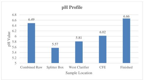
Figure 6: pH samples from Heavener WTP major unit processes on August 28, 2019
