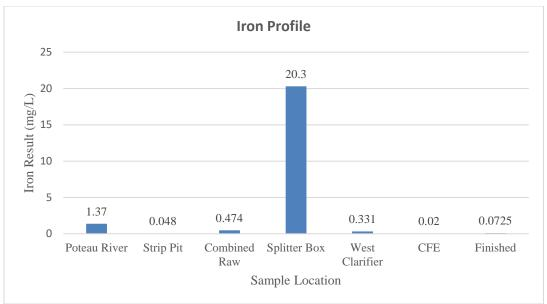
Figure 4: Iron samples from the Heavener WTP major unit processes on August 28, 2019
