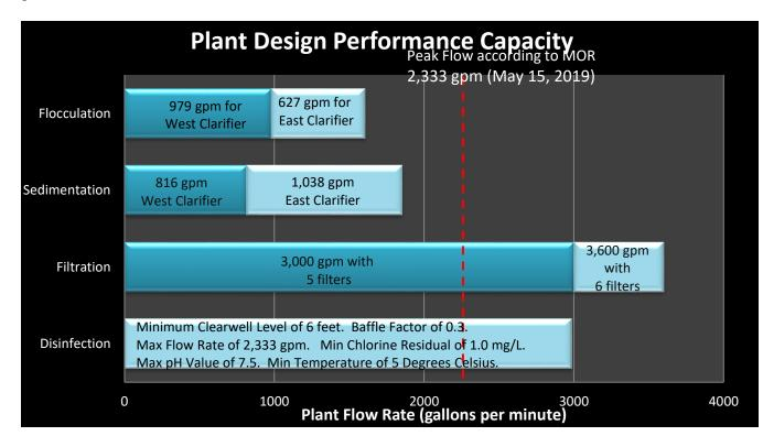
Figure 7: The calculated capacities of each major unit process
